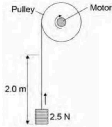
He used the motor to lift a weight of 2.5 N a height of 2.0 m.
