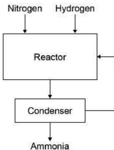
A mixture of ammonia, hydrogen and nitrogen gases leave the reactor.
