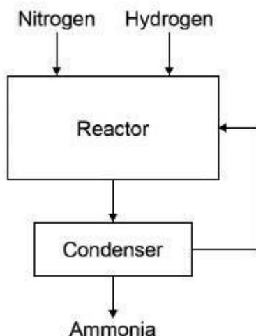
A gaseous mixture of ammonia, hydrogen and nitrogen leaves the reactor.
