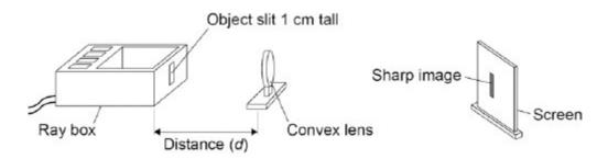
(a) The student measured the magnification produced by the lens by measuring the image height in centimetres.
