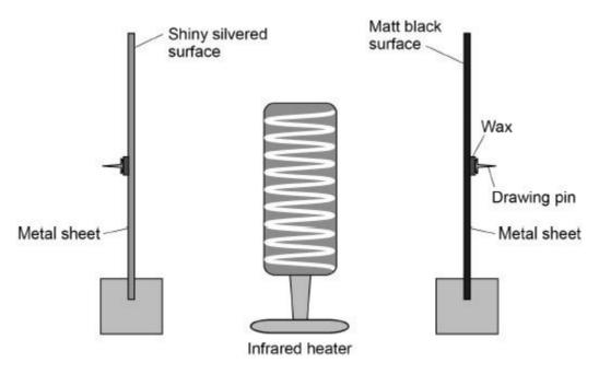
The metal sheets absorb infrared radiation. The wax melts and the drawing pins fall off the surfaces.
