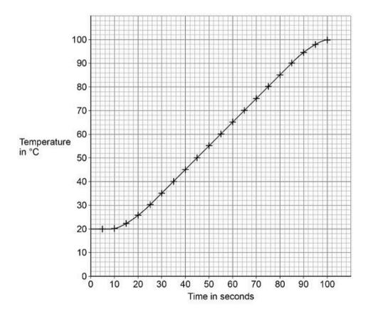
(d) The temperature of the water did **not** start to increase until 10 seconds after the kettle was switched on.
