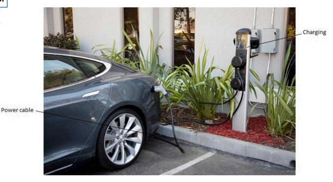
(a) The charging station applies a direct potential difference across the battery of the car.
