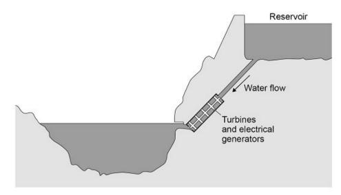
Electricity is generated when water from the reservoir flows through the turbines.
