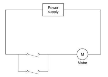
The lift can be operated using either of the two switches. Explain why.
