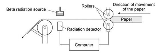
The computer uses information from the radiation detector to change the size of the gap between the rollers.
