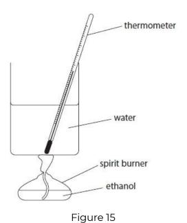
The theoretical temperature rise for burning a given mass of ethanol is 82.4 °C.
