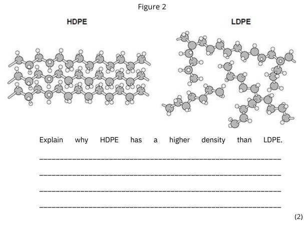
Figure 2 represents part of the structures of HDPE and LDPE.
