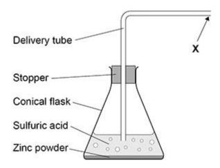
(a) X shows where a piece of equipment is connected to measure the volume of hydrogen gas collected.
