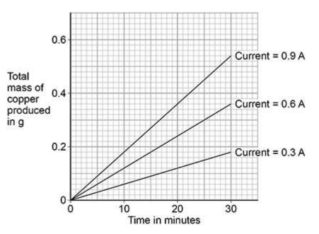
A student correctly concluded that the total mass of copper produced is directly proportional both to the time and to the current.
