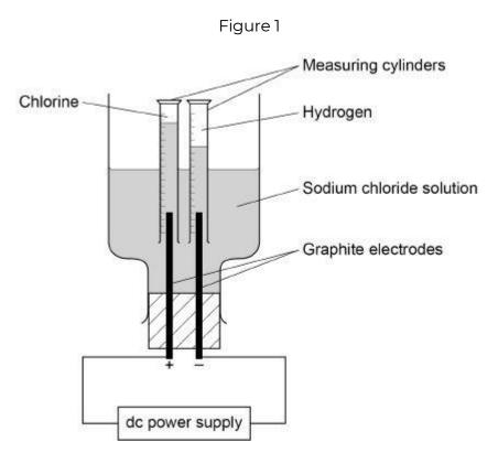
The student measured the volume of gas collected in each measuring cylinder every minute for 20 minutes.
