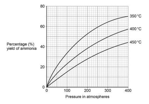
A temperature of 450  $^{\circ}\mathrm{C}$  and a pressure of 200 atmospheres are used in the Haber process.
