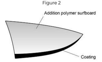
The coating is made from soda-lime glass fibres surrounded by a plastic.
